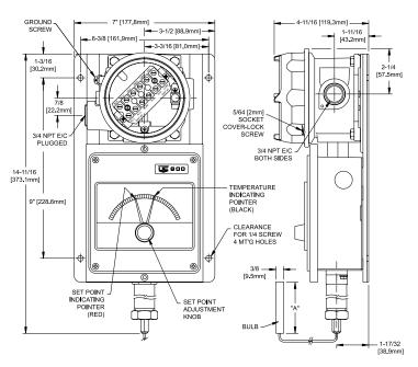
†Type 802 has a second set point indicating pointer (green). Type 800 has no set point indicating pointer.
