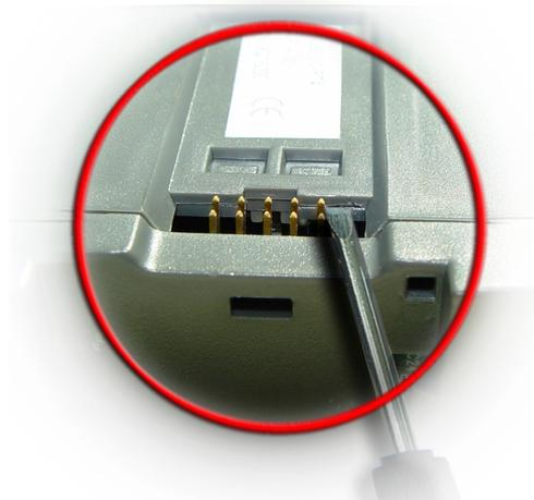
2. Taking care not to damage the cable, open the other side of the device by inserting the blade where shown below, then gently pushing up.
